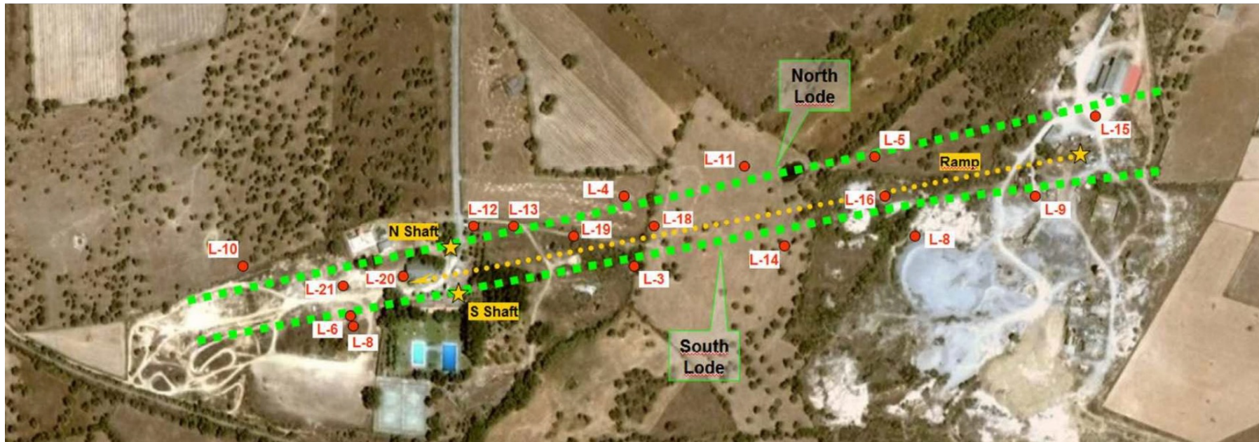
Image surface projection of two vein systems (green) and decline ramp (yellow)
